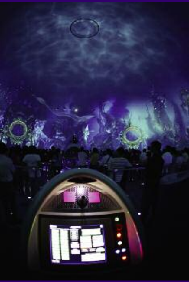
One of two operator control stations—part of the overall Navigator-based show control system.
