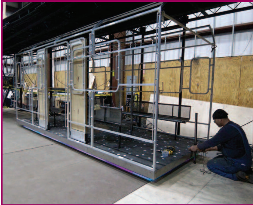
The subway set, built by Hudson Scenic Studio, was one of the show's top challenges.
