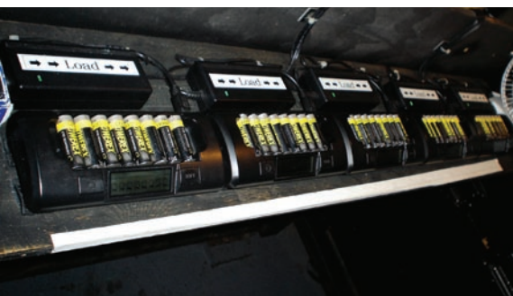
One set of nickel-metal hydride (NiMH) rechargeable batteries recharging for the next showing of Wicked .
