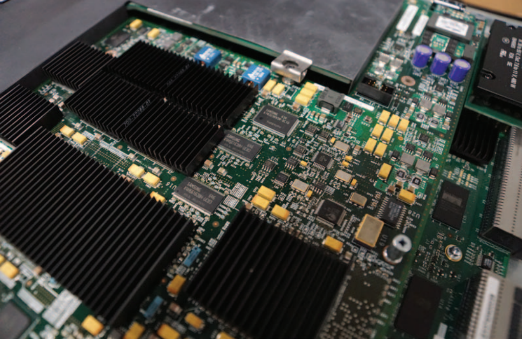
A view inside a high-end router's supervisor engine. Routers like these can handle both IPv4 and IPv6 traffic simultaneously and at high speed.
