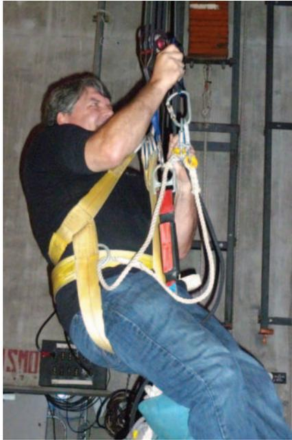
A "rescue cradle" with a block and fall are used to allow a single rescuer to ascend to the victim and then lower them to the ground.
