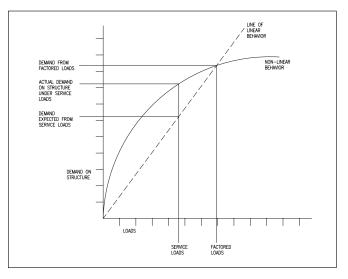
With ASD, the engineer designs for the actual loads that the structure is expected to see. That way, the demands that will be placed on the structure are correct and the designer can then apply the appropriate factor of safety.
