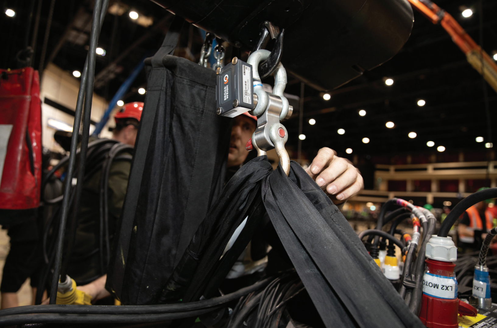
Figure 1 – Broadweigh BW-S475-TL Wireless Load Shackle on The 1975 UK Tour, Motorpoint Arena, Cardiff, UK
