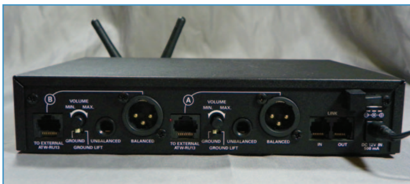
System 10 Pro I/O includes balanced and unbalanced outputs, RJ45 connectors for external receiver unit connection, and RJ12 connectors for system linking.
