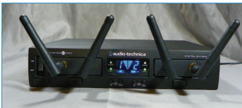
A half-rack chassis holds two receiver units.
