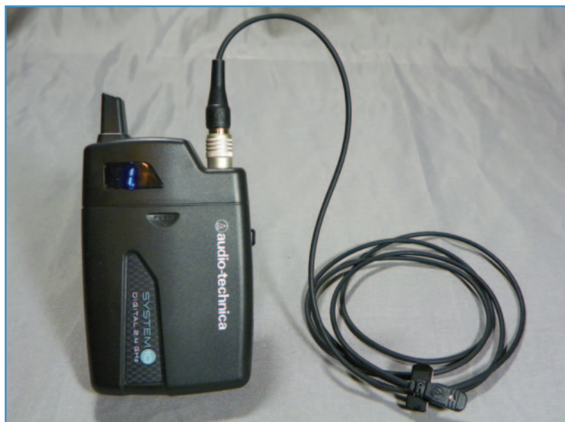
UniPak body pack transmitter with MT830cW omnidirectional lavalier mic.
