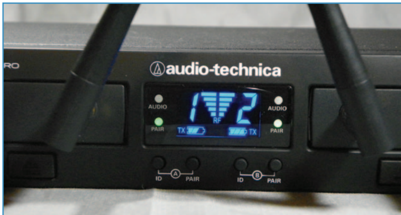
The display indicates channel, RF level, battery level, pairing, and audio present. The buttons are for ID selection and pairing.
