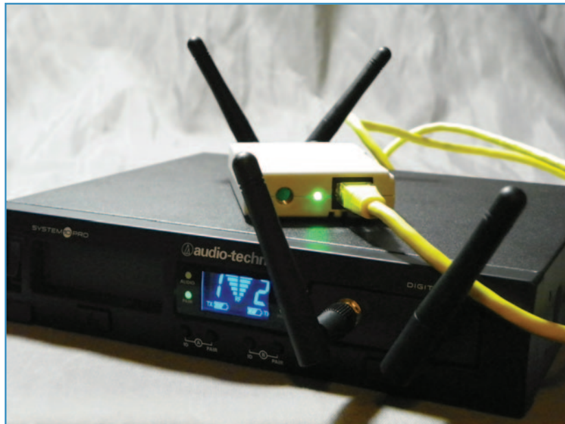
Receiver with Ethernet cable plugged in for remote location.
