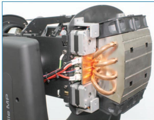
Figure 2: LED array and cooling.
