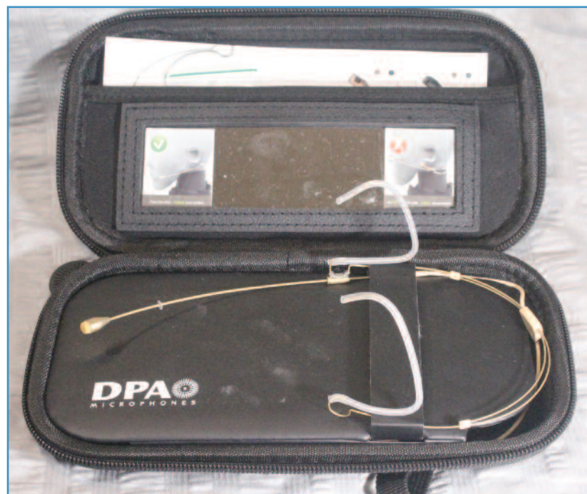
DPA 4466 CORE omnidirectional headset mic in the storage case (that's a mirror in between the pictograms to check placement and fit).
