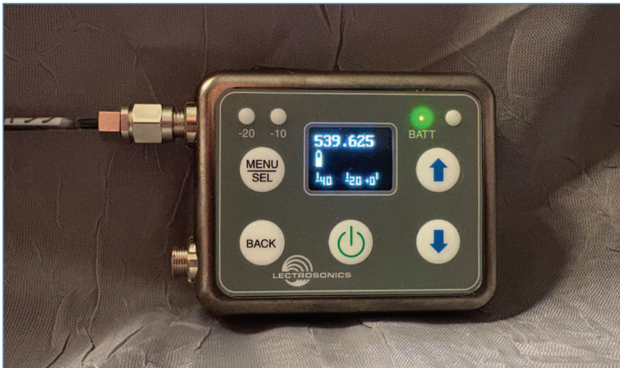
DSSM front control panel.
