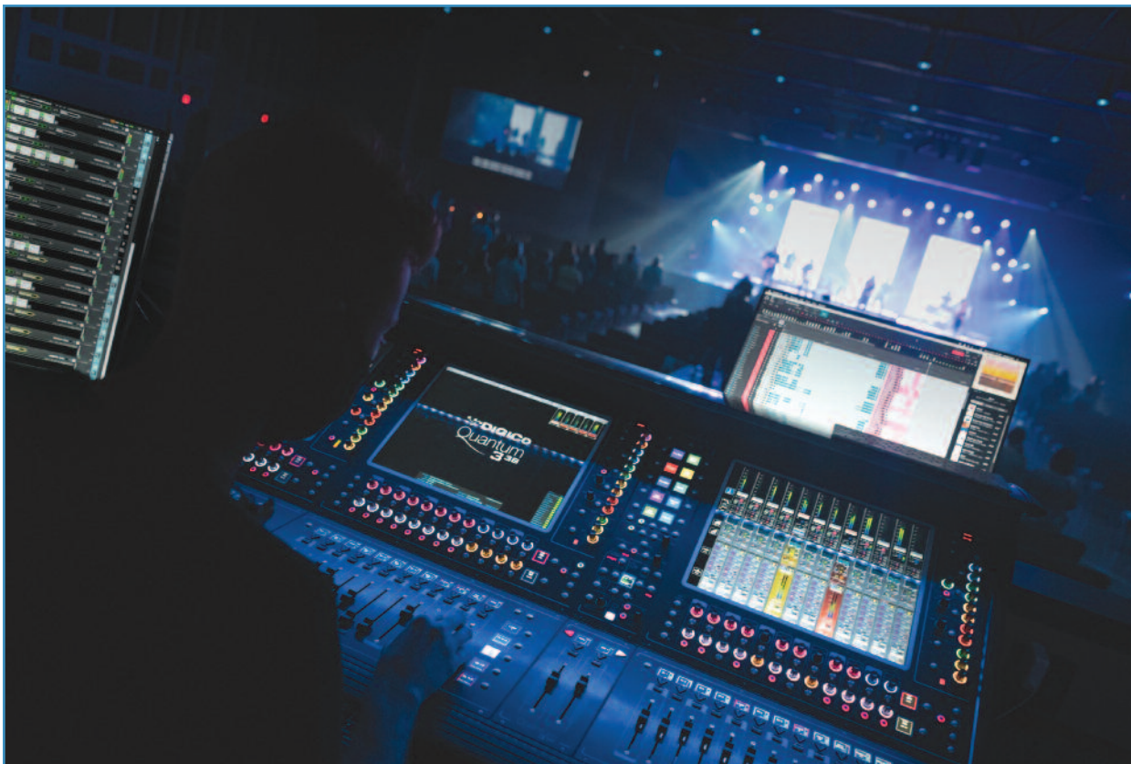
The 338 has a trio of 17", 1,000-nit, high-brightness multitouch screens, with the meter bridge and soft quick select buttons displayed on each screen,
