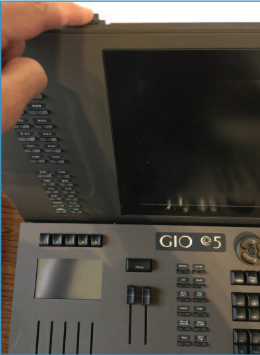
The multi-touch LCD display articulates with the touch of a button. It can fold flat for transportation or it can be angled for use while you are standing or sitting.
