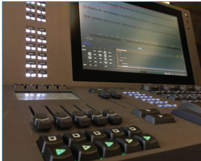
The Gio @5 shares a lot in common with the full-sized Gio console, including its backlit control keypad and navigation keys. The Gio @5 has a 17" touch screen, five motorized playbacks and load buttons, and 24 customizable hardkeys.
