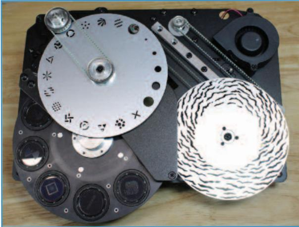
Figure 10: Gobo module, effects wheel out.
