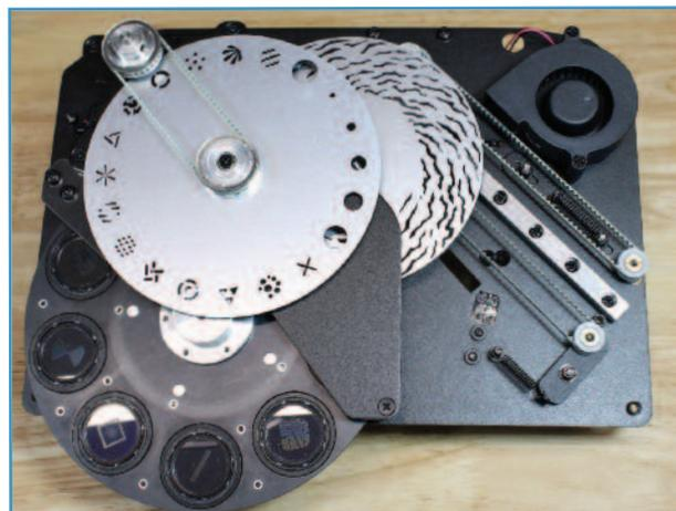
Figure 9: Gobo module, with effects wheel in.
