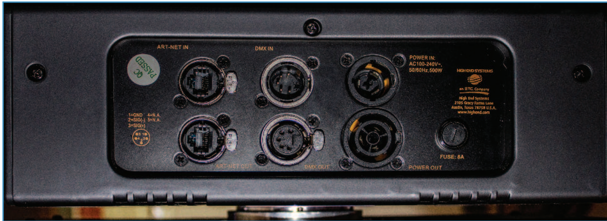
The connector panel includes two Ethernet connectors (input and output), DMX in and out, and etherCON True1 input and output. The current draw at 120V is about 3.6A, which means you could connect four fixtures on a 20A circuit and still have some overhead.
