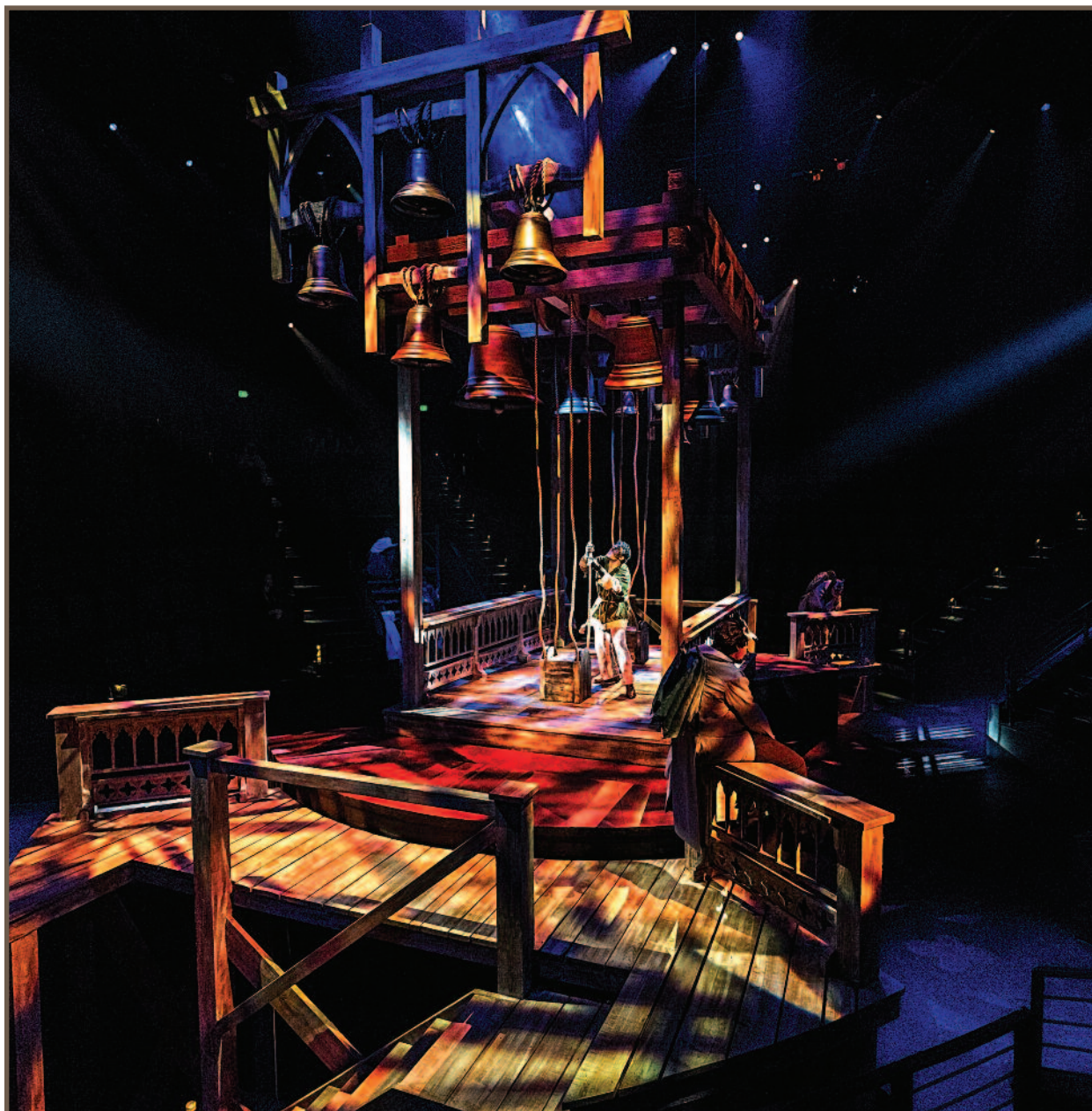
The Hunchback of Notre Dame. The lighting rig combines ETC conventional and LED units with High End Systems SolaFrame Series automated units and Robert Juliat followspots.
