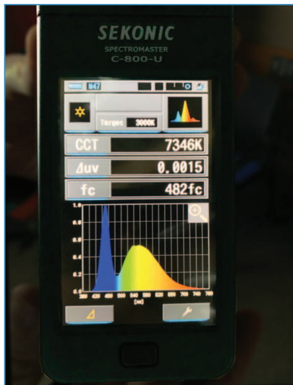
At a throw distance of about 30', it produced a spot about 7' in diameter with an illuminance of 482fc (5188 lux).
