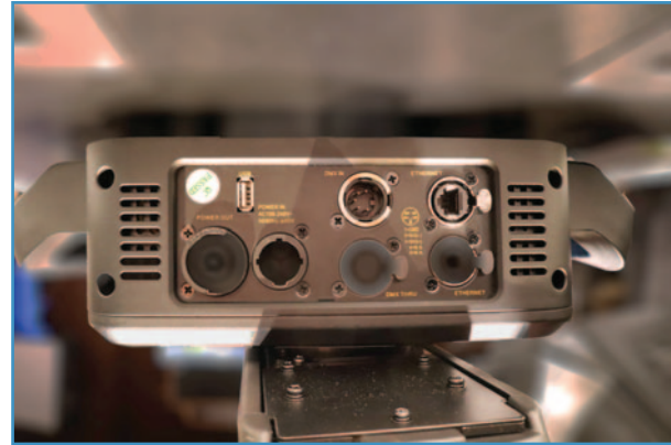
The connection panel has both XLR (DMX in and thru) and Ethernet (in the thru) connectors, and the fixture can accept Art-Net or sACN. It can also act as a gateway (or node) with an Art-Net or sACN input and DMX output, and it works with RDM.
