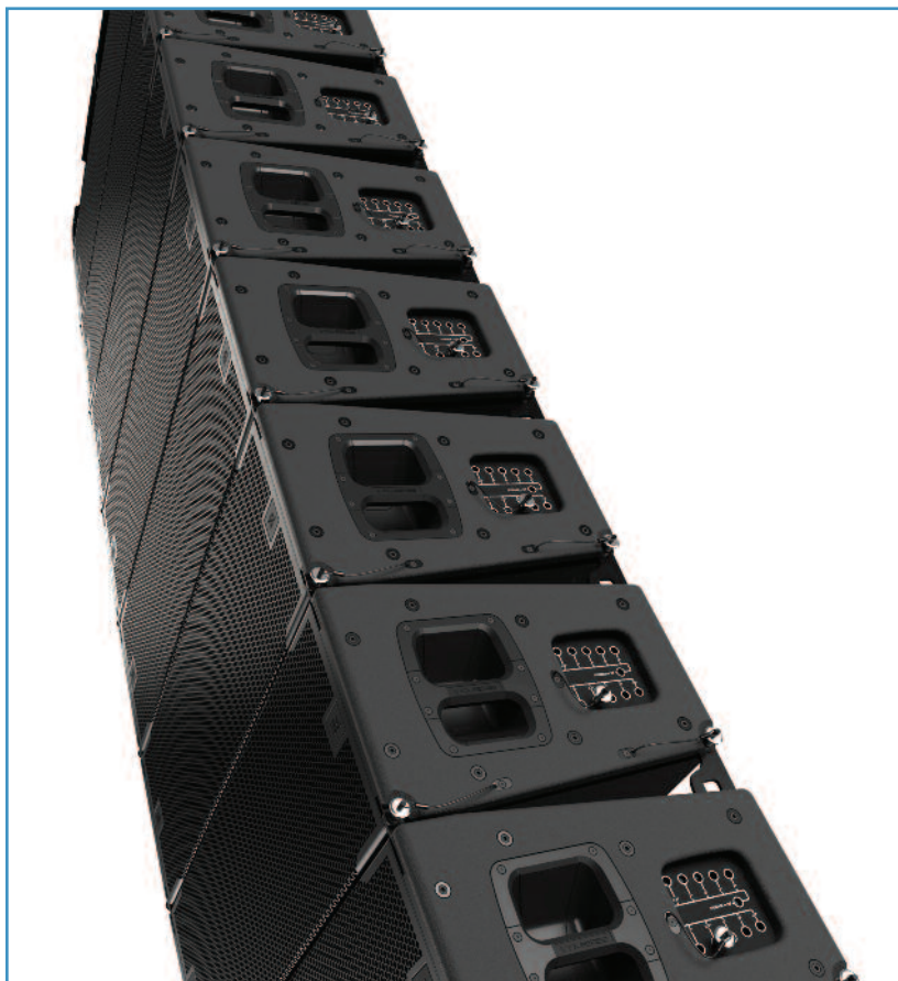
The all-new A12 rigging features a tension-only, auto-locking system, with 0.25° to 10° options and a single hinge point for improved accuracy.
