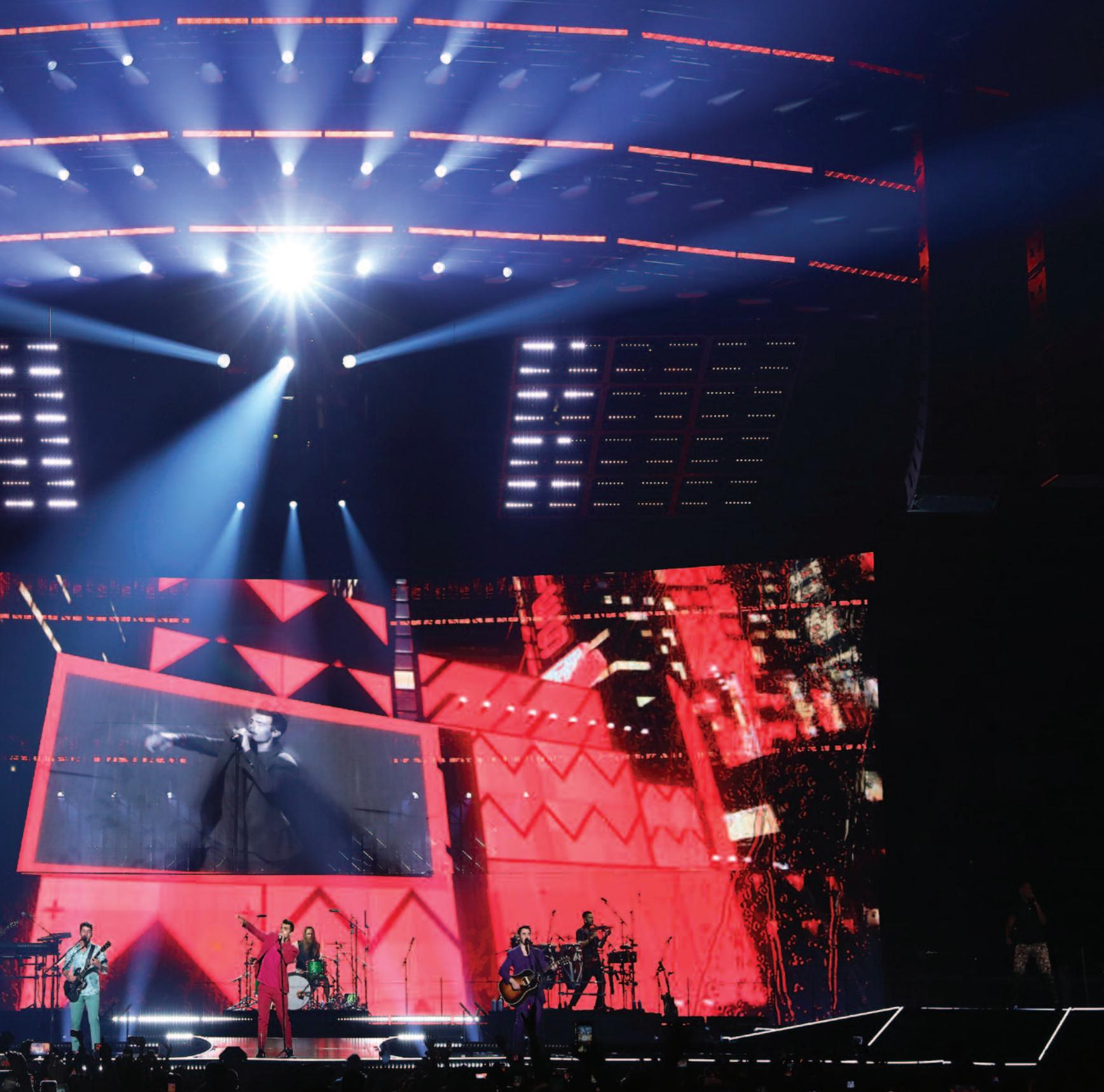
Reardon created a rig featuring three curved front trusses filled with Claypaky Scenius Profiles and lined with GLP Impression X4 Bar 20s.
