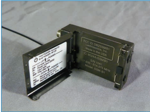
Transmitter with hinged door and battery pack removed.
