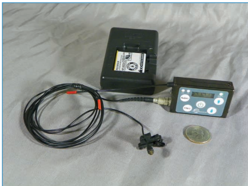
The SSM Micro transmitter with a DPA 4061 mic and battery pack charger unit. The quarter is in the picture for size reference.
