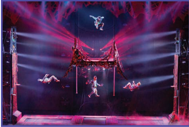
Two 96' overhead tracks have two acrobatic trolleys each for the moving artists, some of whom fly over the audience.
