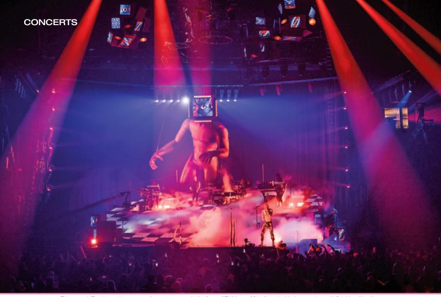
This spread: The Internet looms over the upstage area in the form of TV Man, a 29'-tall, matte black, puppeteered inflatable with articulating limbs and an LED tile face. "All the R&D work was done with the Inflatable Design Group," Gorleski says. Movements are handled by SGPS winches and a Raynok control system.
