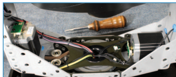
Fig. 17: Pan and tilt motors.
