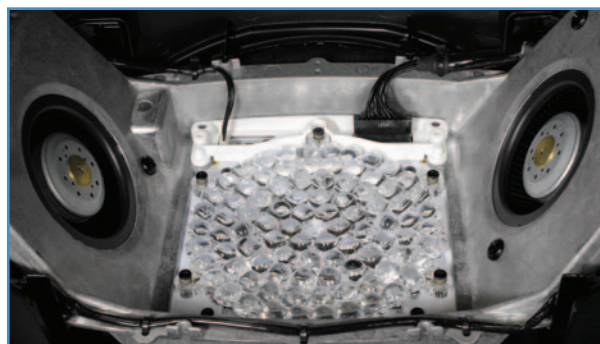
Fig. 2: LED lenses and cooling.
