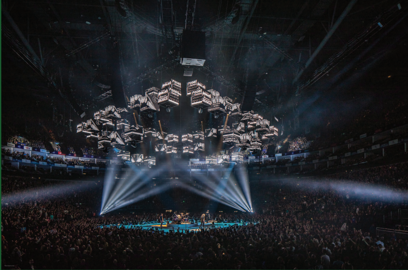
The cubes pose a rigging challenge, due to their weight and the fact that they're automated.
