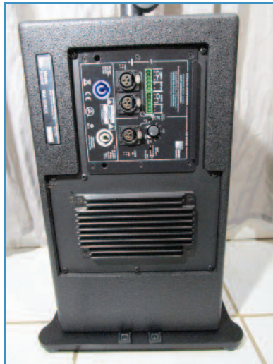
MM-10ACX subwoofer and system I/O.
