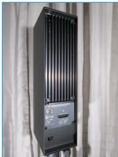
UP-4Slim Phoenix input connection and heat sink.
