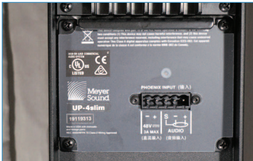
UP-4Slim Phoenix input connector.
