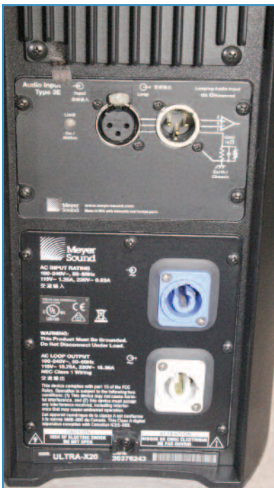
I/O panel with looping XLR and PowerCon connectors
