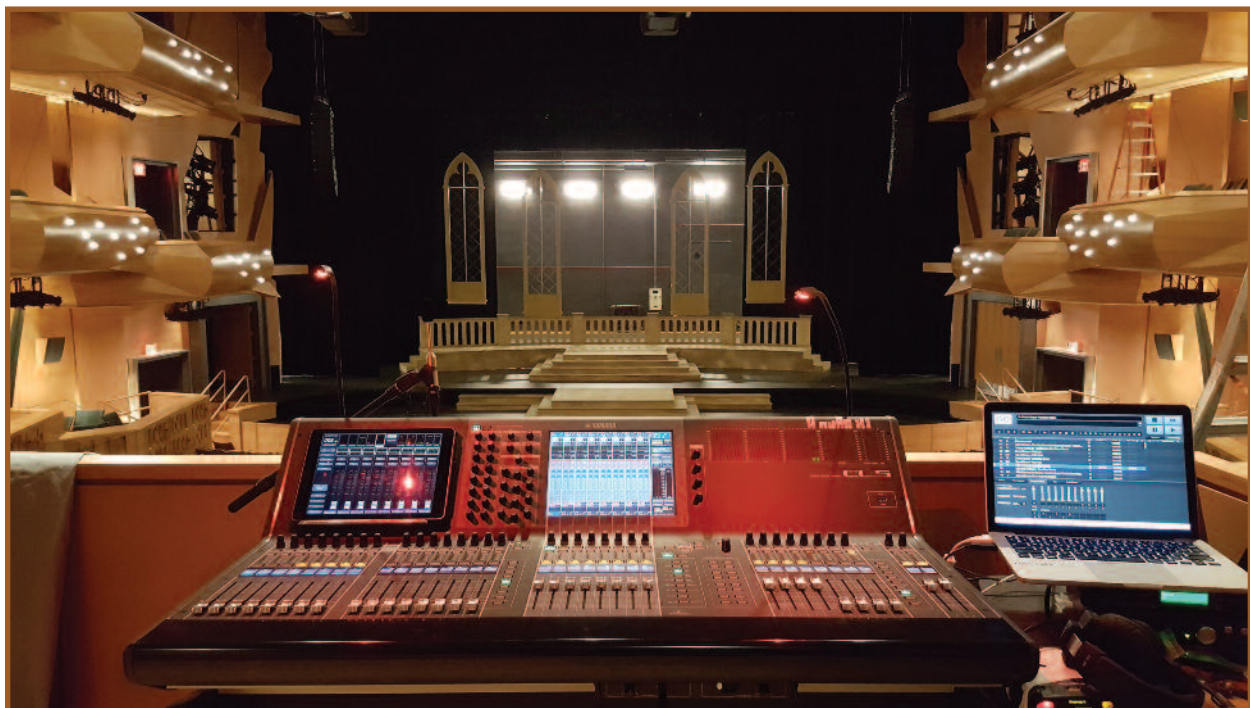
A Yamaha CL5 digital console, with an MB200 meter bridge and three Dante-MY16-AUD cards, was specified for the front of house.
