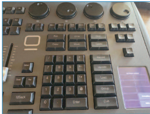
The console runs Onyx software, which is well-developed and has features like the Onyx Remote software app for iPhone to provide wireless control for remote focusing, remote cue execution, and fixture testing.
