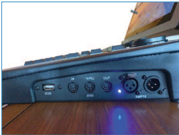
Features include USB; MIDI in, out, and thru; SMPTE, and other hardware features found on full-sized consoles, but in a compact form factor.
