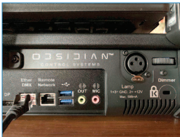
The NX 2 can output 64 universes of DMX via four DMX ports and one Ethernet port.
