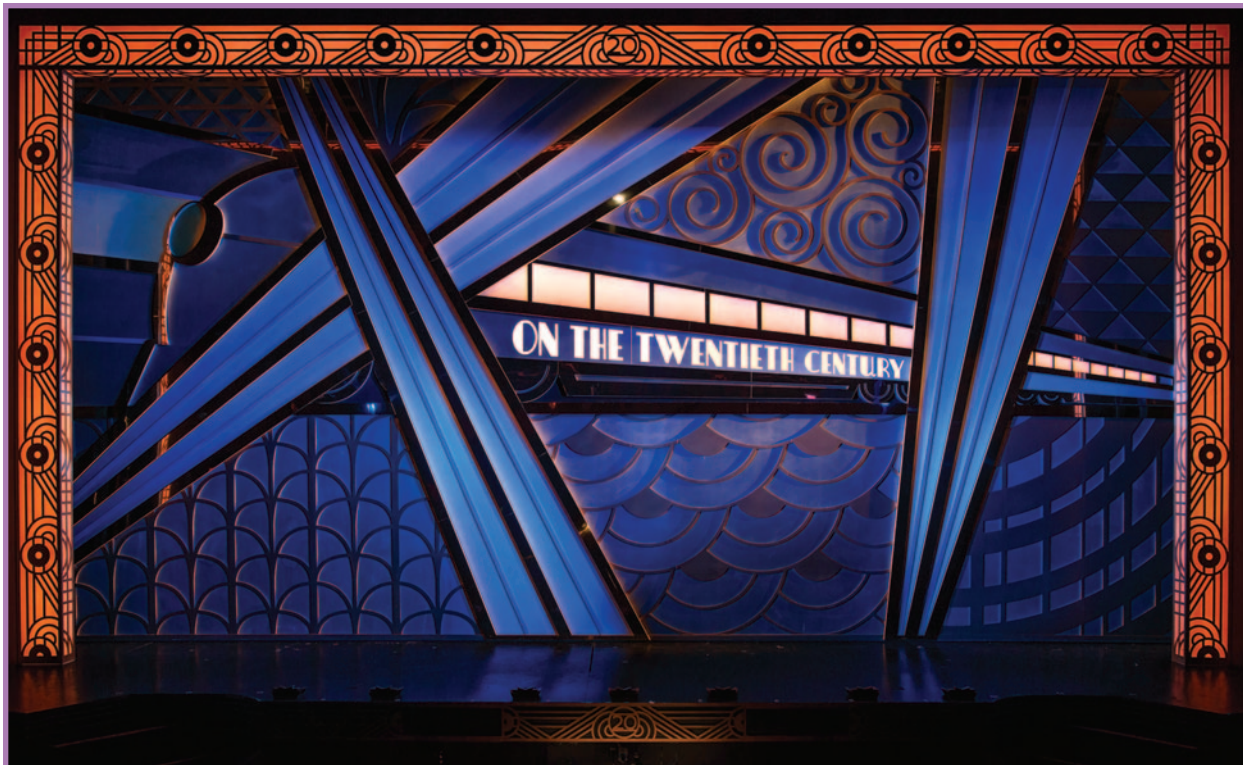
The show curtain is a forced-perspective view of a train and powerful beams of light; the surrounding portal is a lightbox filled with LED tape.
