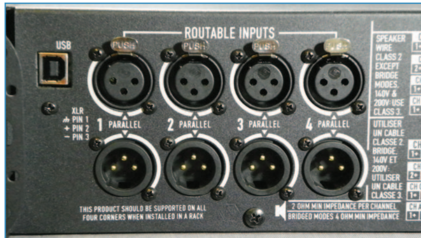
The rear panel I/O includes four routable, paralleled inputs and USB port (above), and six Neutrik NL-4 loudspeaker output connectors (center).
