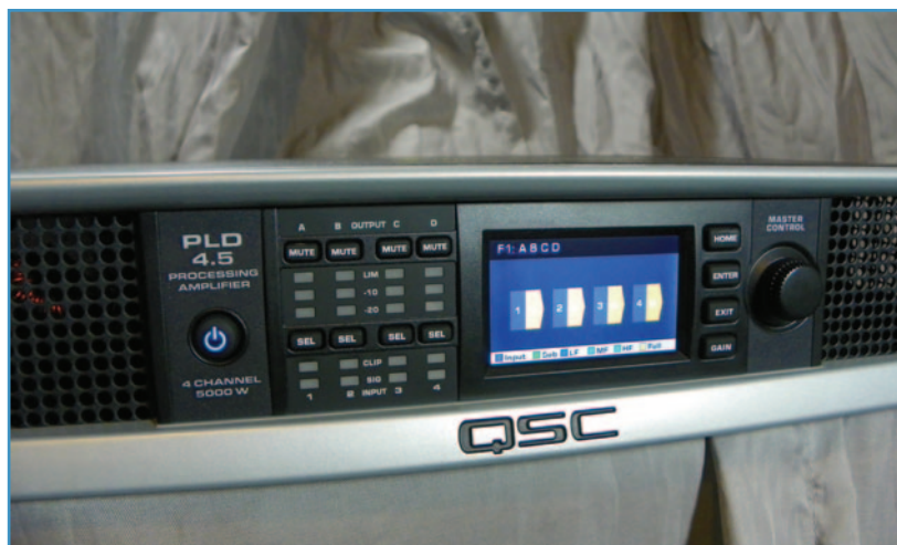
The graphic display provides control, status, and operational information.
