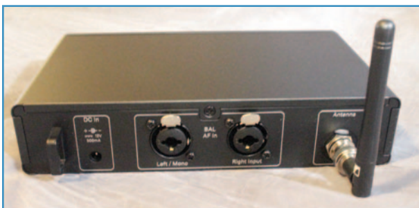
XSW transmitter rear panel. The inputs are electronically balanced XLR 1/4" combo sockets.
