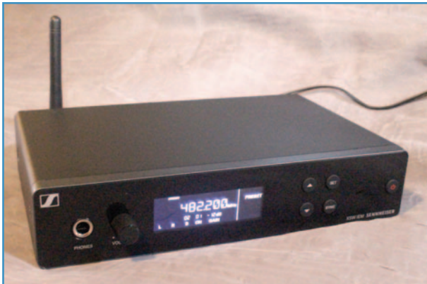
XSW transmitter front panel. The basic controls provide a fair amount of functionality.
