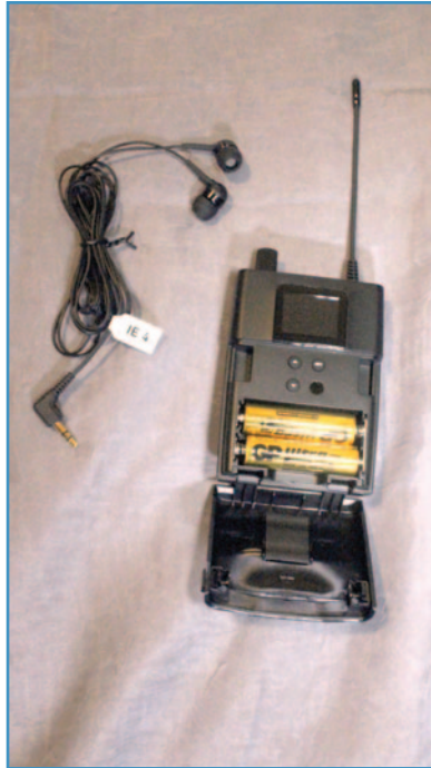
XSW receiver pack battery and control access.
