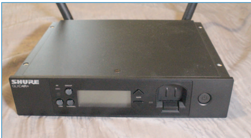
Shure GLX-D4R receiver front panel; note battery charging port on right.
