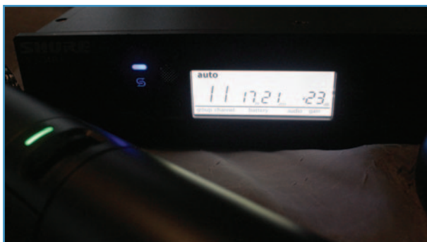
GLX-D4R receiver display with sync indicator.
