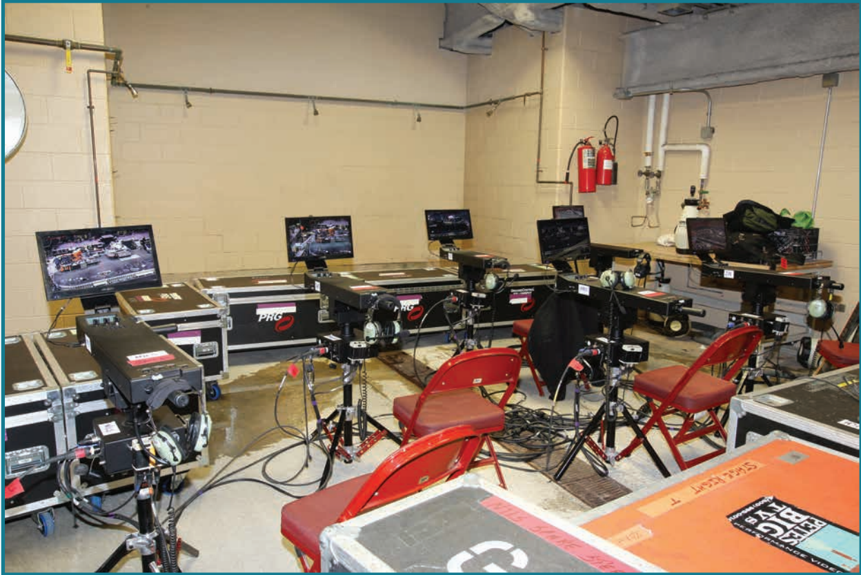
Above and below: PRG's GroundControl system eliminates the need for local spot operators to climb up and down 40'.
