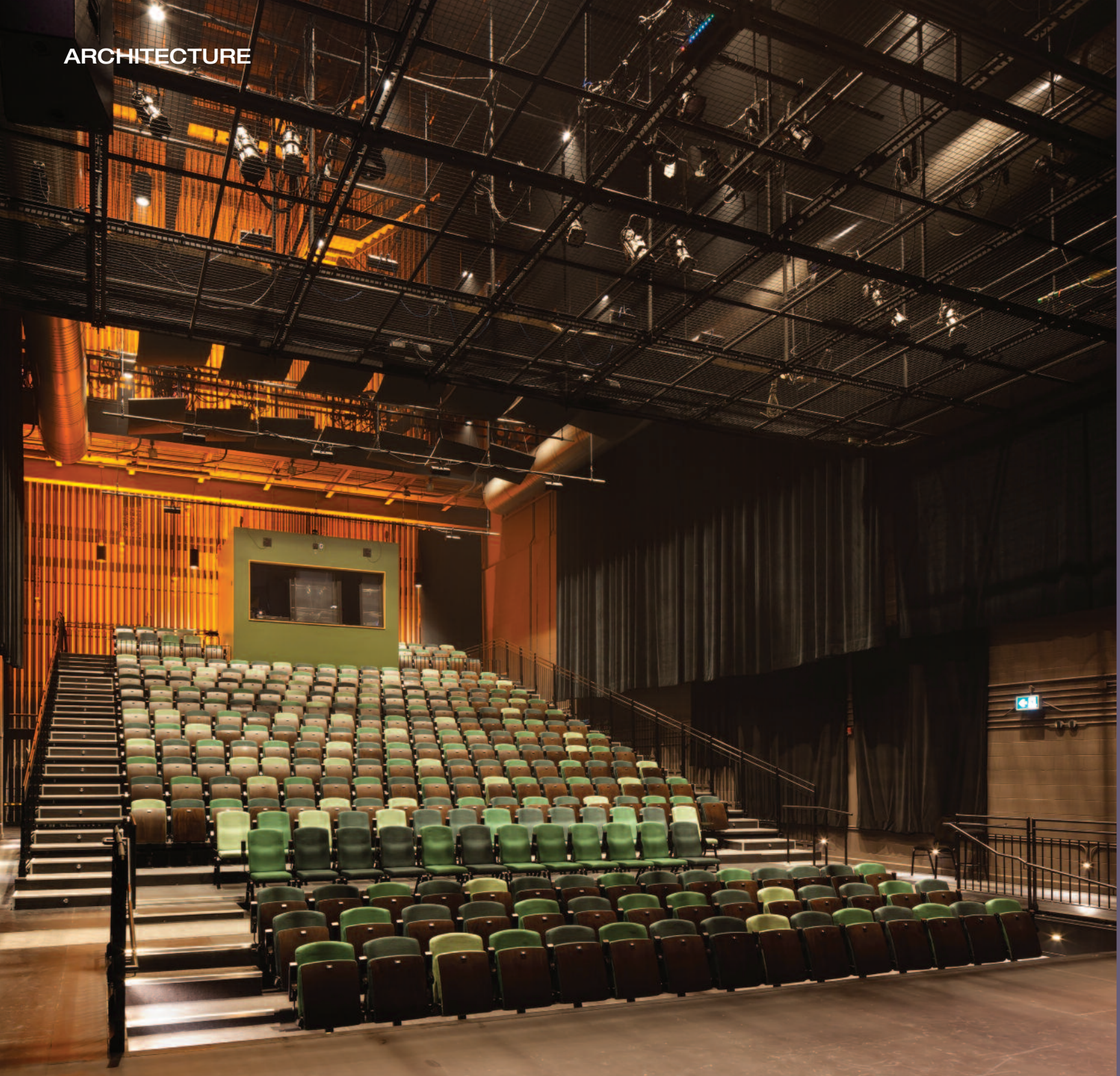
The 296-seat Greenwin Theatre, built entirely on the former Main Stage, features retractable seating and a tension-wire grid.
