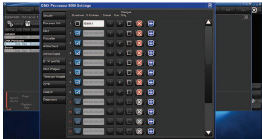
Many automated lighting consoles default to broadcasting Art-Net protocol. If you configure it to unicast by deselecting the broadcast option, then it will use less bandwidth and produce less network congestion.
