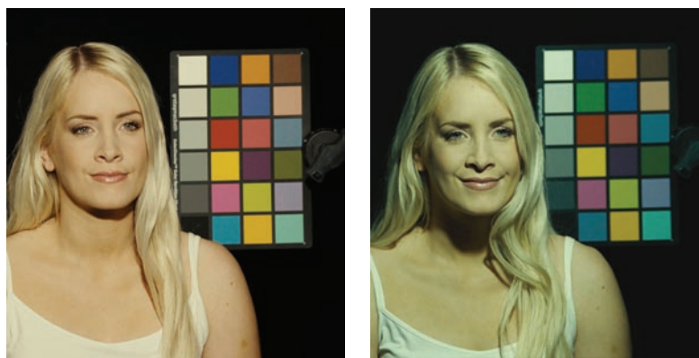
Figure 9 – A subject lit with two different LED sources. The source on the right has a shift towards green, which is more readily apparent on skin than on the color chart.
