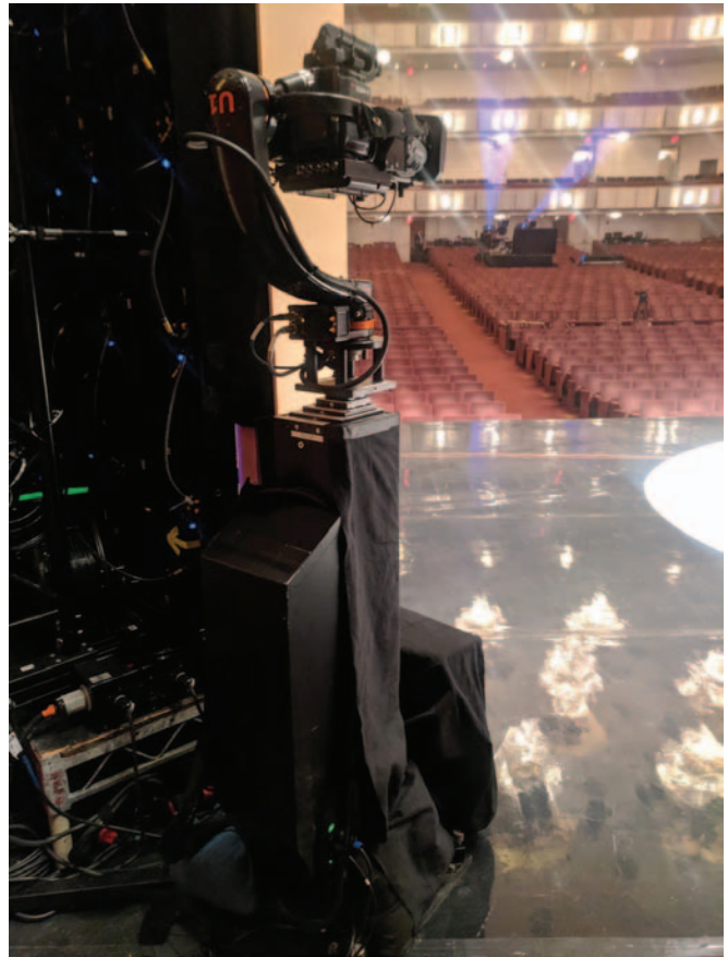
A robotic camera in the wings takes up less space than a human camera operator and is less likely to upstage the talent.
