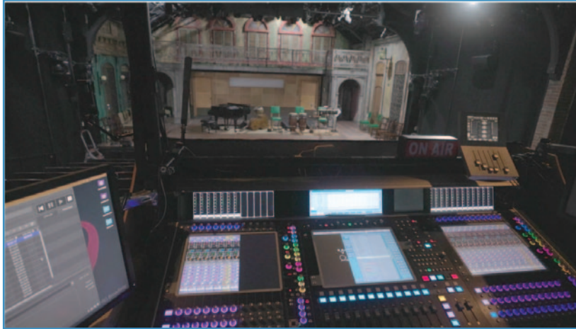
Control was provided by a DiGiCo SD7 Quantum console, chosen, Dean says, “because we needed to do a lot of tricks, a lot of grouping, and a lot of bussing.”
