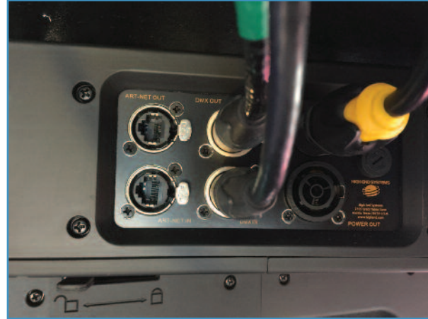
A built-in two-port network switch allows the fixture to accept both Art-Net or sACN directly, and users can daisy-chain the Ethernet cables.
